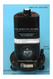
Cat Item **Type** AP-731D D ARSONAL Galvanometer with scale leveling screws coil adjustable
