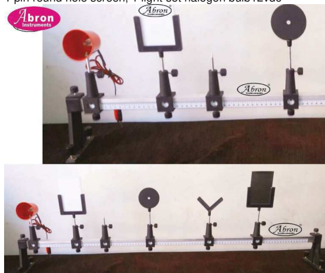
AP-839M5 optical bench single Aluminium pipe with scale 150cm with riders
